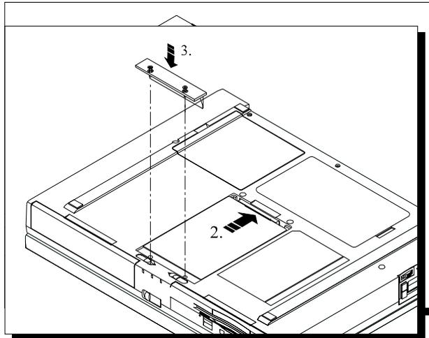
**Installing the HDD module (B)**
