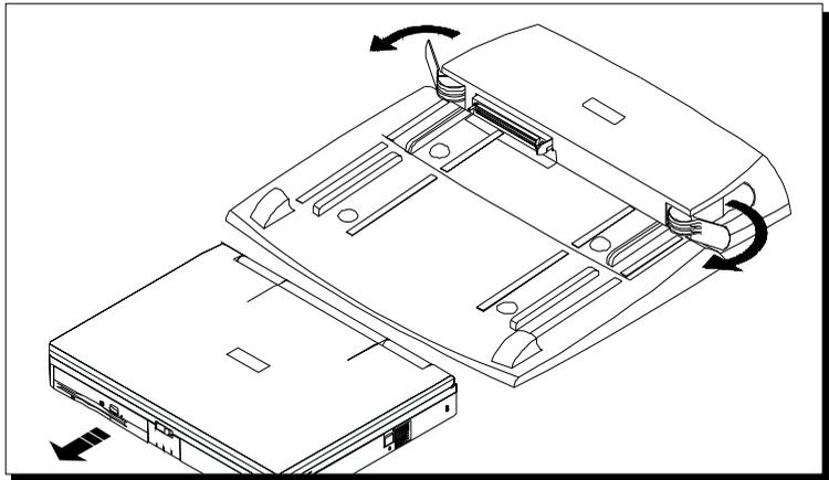
*Figure 6-10: Removing the Notebook from the I/O Replicator*
