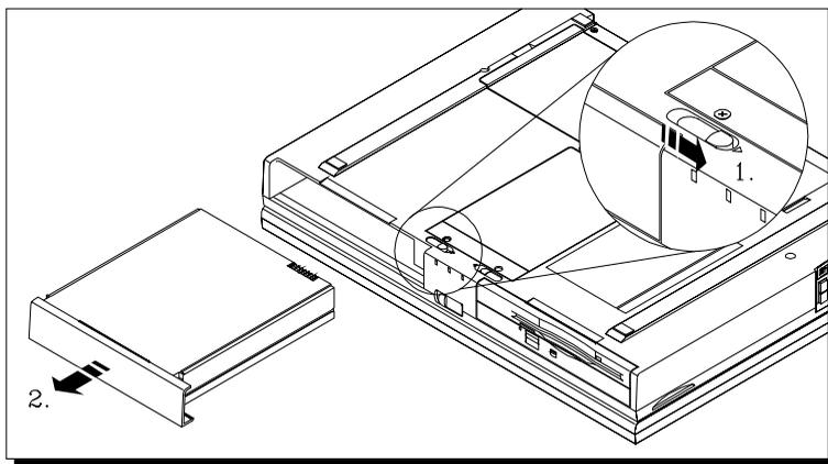
**Figure 5-4: Removing the Battery Pack**
