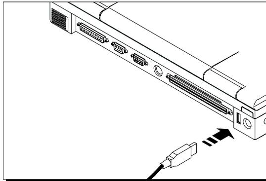
*Figure 4-6: Connecting a USB Device*
